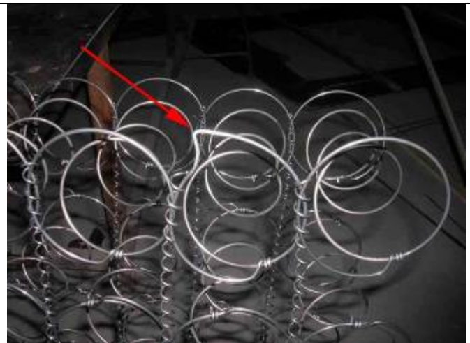
c.2. the spring was deformed
